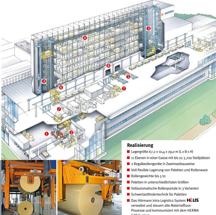
Roll portal with intermediate storage positions for production supply.
