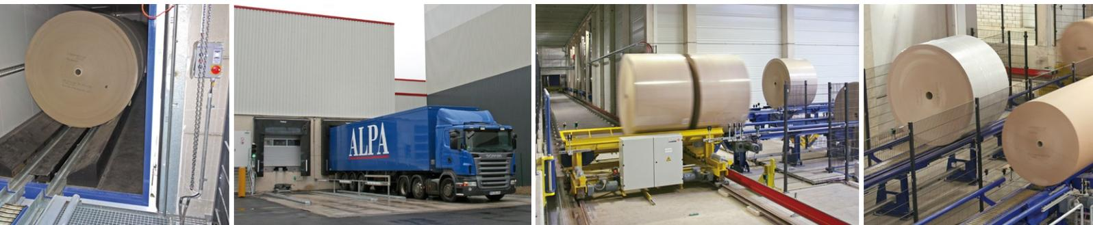
The project includes rack steel constructions, S/R machines, conveyor systems, fire preventions, fully-automated truck loading stations with two special trailers including overall warehouse management, plant control and plant visualization.
